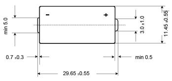
Dimensions are in millimeters and include label.
